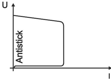
**Anti-stick prevents the electrode from annealing.**
